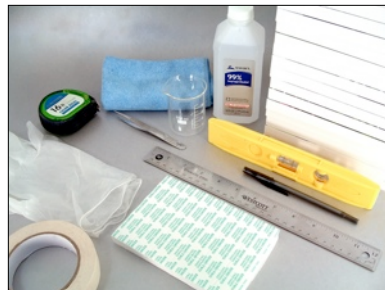
PIC 1-1: Tape measure, tweezers, cleaning supplies, poster panels, level, pen, ruler, adhesive blocks, tape, gloves.
